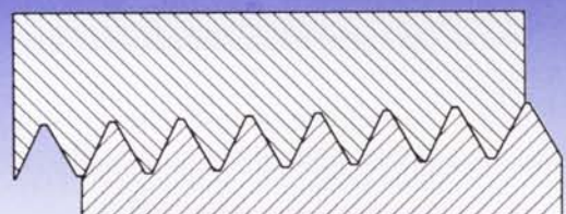
Figure 6 Taper to taper NPT threads
